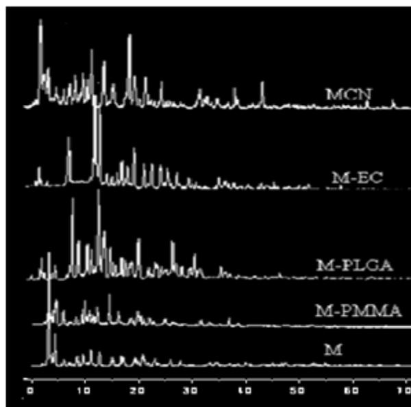
Figure 5: XRD of polymeric nanoparticle, polymer and drug
