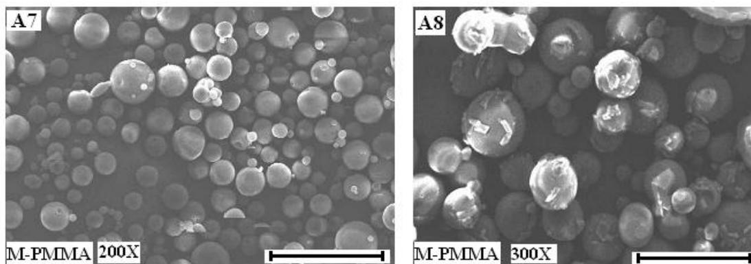
Figure 2: A7- A8 was SEM images of Metformin polymeric nanoparticle. Scale bar indicates 500nm.
